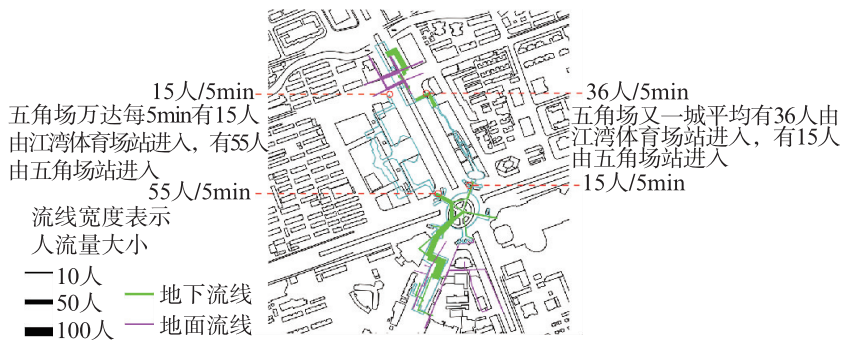
图7 从两个地铁站点进入各综合体的人流情况 Fig.7 Passengers' flow from two metro stations to different mixed-use complexes 资料来源: 作者自绘.
