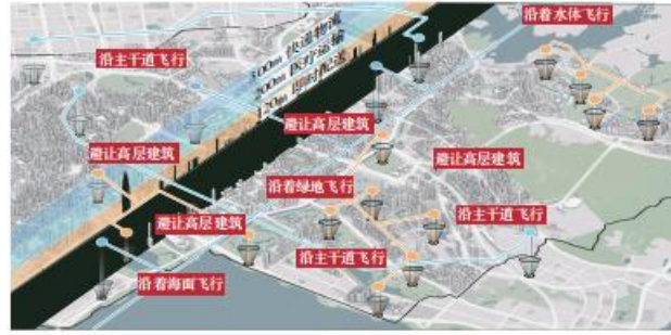
Fig.5 Diagram of low-altitude drone delivery routes in 3D environments in Nanshan District, Shenzhen
