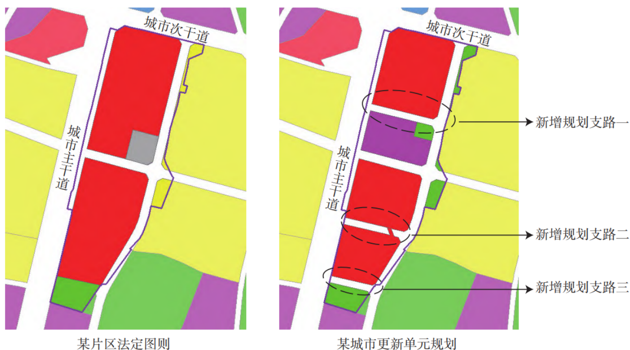
Figure 4. Comparison of planned roads in a renewal-unit plan and the corresponding statutory plan
