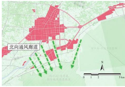
Fig.7 Reserving ventilation corridor through the de- lineation of urban growth boundaries Source: China Academy of Planning (Beijing) Planning and Design Co. Dunhuang spatial master plan (2021-2035) phase results ③ , 2020-2023
